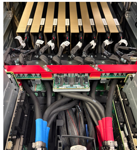
JetCool's Cold Plates for NVIDIA RTX PRO 6000 GPUs
